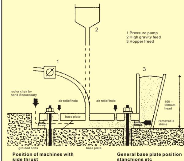
Where the thickness of grout is greater than 50mm, the grout may be bulked out with clean single sized aggregate. However, we have other products, including Five Star Repair Concrete, which may be more suitable. Please contact our Technical Department.
